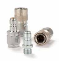
Robust design with small dimensions. Series 1100 is used mainly for applications in the area of compressed air and liquids. Optimally suited to smaller pneumatic systems and to compressed air tools with a consumption of up to 900 litres per minute. Coupling systems with two-hand operation, i.e. both hands are required when connect/disconnect.
