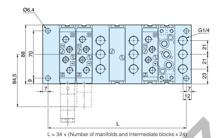
Connection block L and intermediate blocks L and T can be turned so that connection can be made from above or below.
