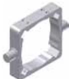
Intended for articulated mounting of cylinder. The trunnion is factory-fitted in the centre of the cylinder or at an optional location specified by the XV-measure – Combined with pivot brackets for MT4.
