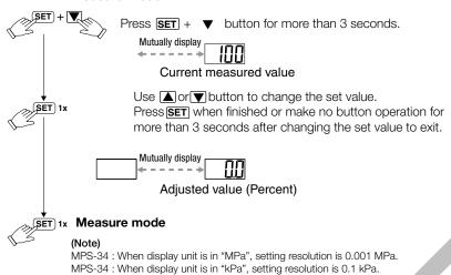
This function eliminates slight differences in the output values and allows uniformity in the numbers displayed. Displayed values of the pressure sensor can be calibrated to within ±5% for MPS-P34 and ±2.5% for series MPS-V34.
