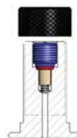
Model of valve stem integrated 5/8" 18 UNF (D)
