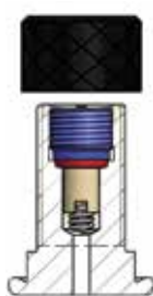
Model of valve stem integrated 7/8"14 UNF (C)
