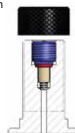
Model of valve stem integrated 5/8" 18 UNF (D)
