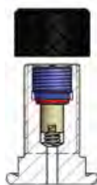
Model of valve stem integrated 7/8"14 UNF (C)
