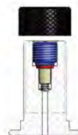
Model of valve stem integrated 5/8" 18 UNF (D)
