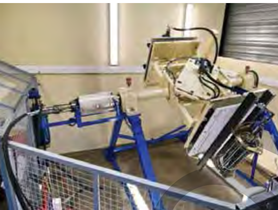
Accumulator test bench for wind turbine application.
