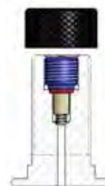
Model of valve stem integrated 5/8" 18 UNF (D)
