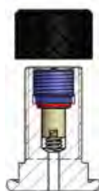
Model of valve stem integrated 7/8"14 UNF (C)
