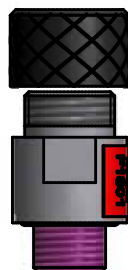
Model of valve stem 5/8" 18 UNF (A)
